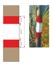
Horizontal or ground stripe marking is a mark consisting of three stripes, each 3 cm wide and with a length of 20 cm. This marking consists of a central white stripe and two outer red stripes. Ground stripe marking is placed in the direction in which teh path runs. In places where there is an intersection of the path, In places where there is an intersection of the path, intermitten marks are in the direction of the path are arranged to follow the direction.
